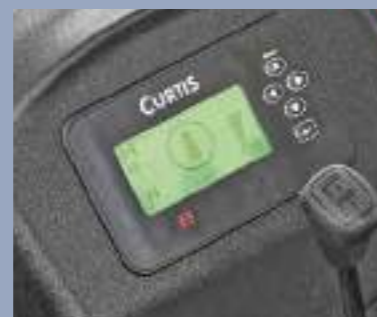
Instrument can display the steering angle and direction Synchronously
